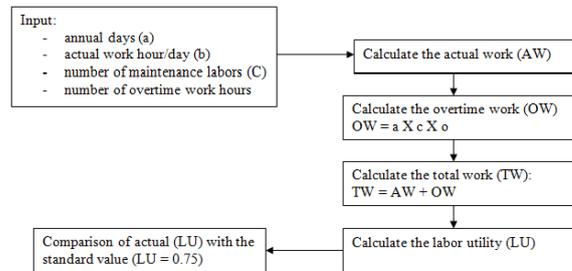
Figure 6: Calculation procedure of Labors utility (LU) pointer
