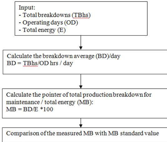
Figure 7: Calculation procedure of production breakdown for maintenance
