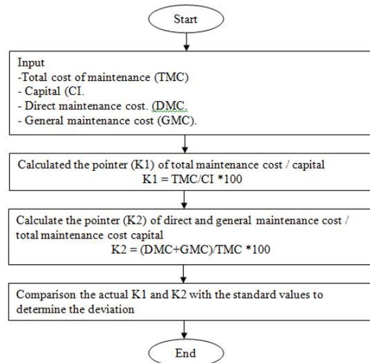
Figure 5: Calculation procedure of costs factor pointers.
