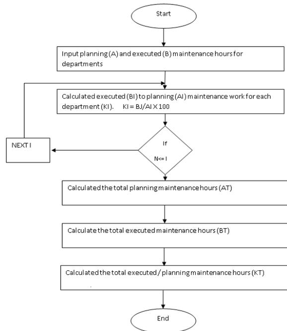
Figure 3: Calculation procedure for executed / planning maintenance hours.
