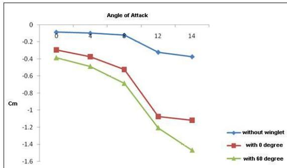
Figure 6.a: Pitching moment coefficients for the wing model (Reynolds number  $1.66 \times 10^5$ ).
