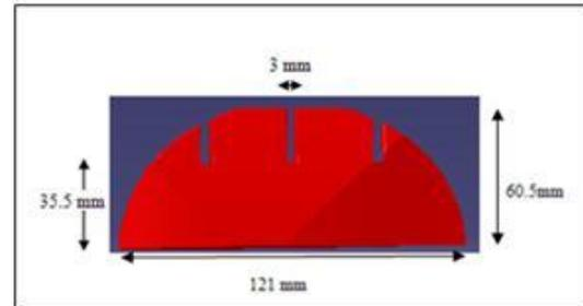
Figure 1: Geometry Characteristic of Bird Feather like Winglet from Top View.
