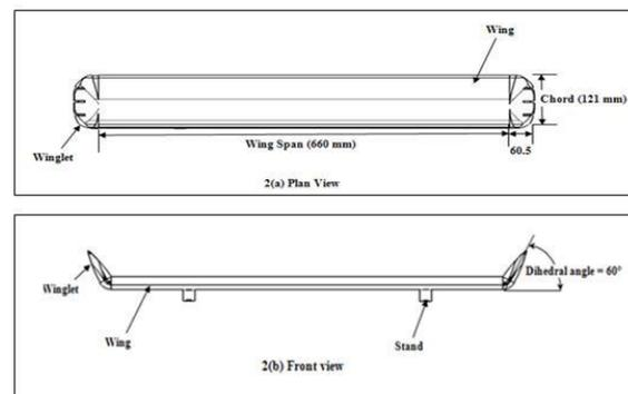
Figure 2: Rectangular Wing with Winglet Inclination using Adapter.
