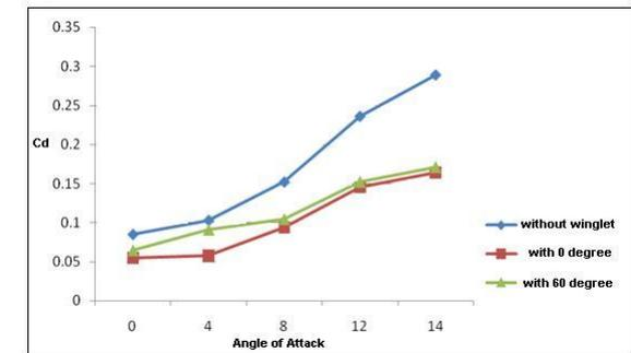
Figure 4.b: Drag coefficients for the Aircraft wing model (Reynolds number  $2.08 \times 10^5$ )
