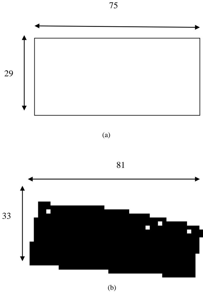
Figure 9: Exploration with real robots. (a) is the environment to be explored, (b) is the generated map. The dimensions shown are in centimeters.
