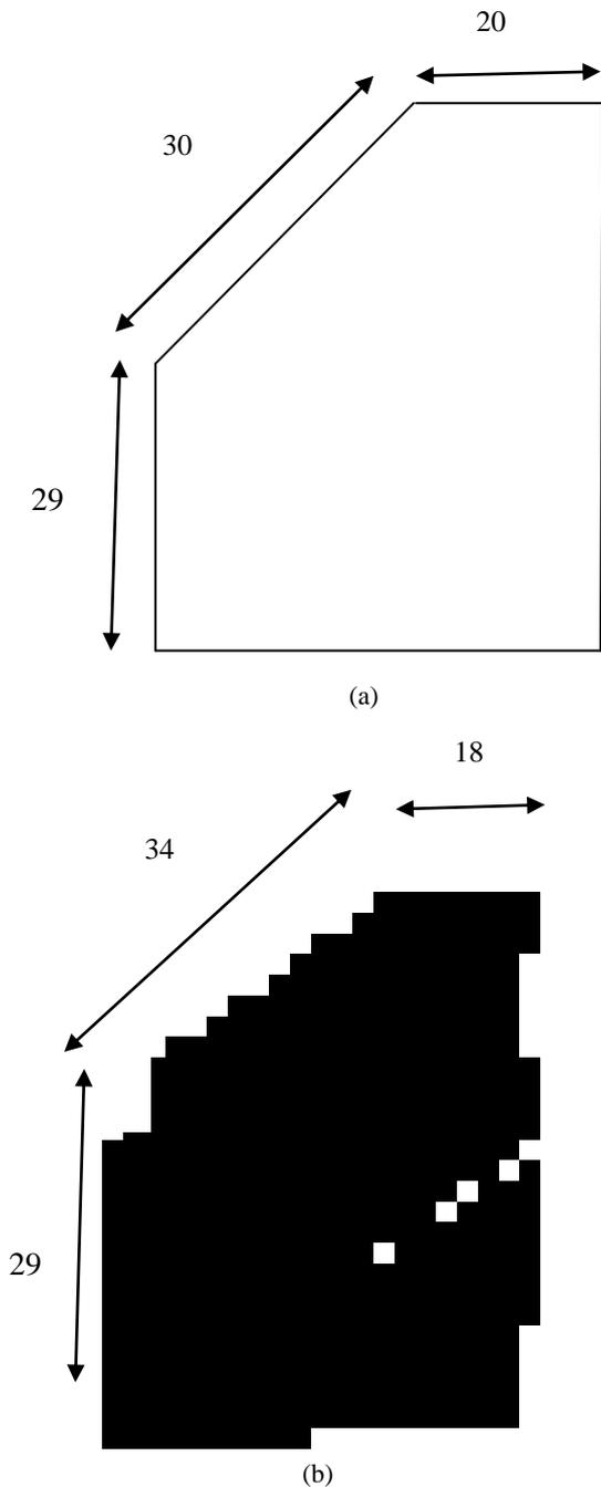
Figure 8: Exploration with real robots. (a) is the environment to be explored, (b) is the generated map. The shown dimensions are in centimeters
