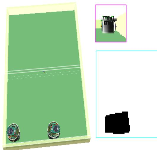
Figure 4: Wall-following exploration experiment with camera image and the constructed map thus far
