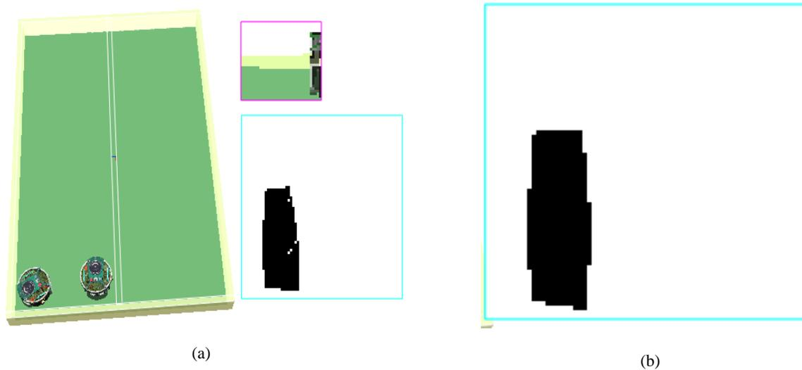
Figure 3: (a) Wall-following exploration experiment with camera image and constructed map thus far (robot speed is 300cm/minute), (b) Map generated at speed of 200cm/minute
