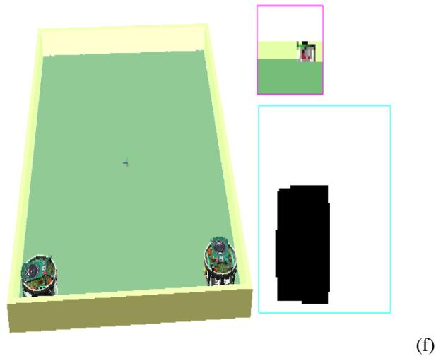
Figure 2: Wall-following exploration progressive snapshots with camera image and the constructed map thus far
