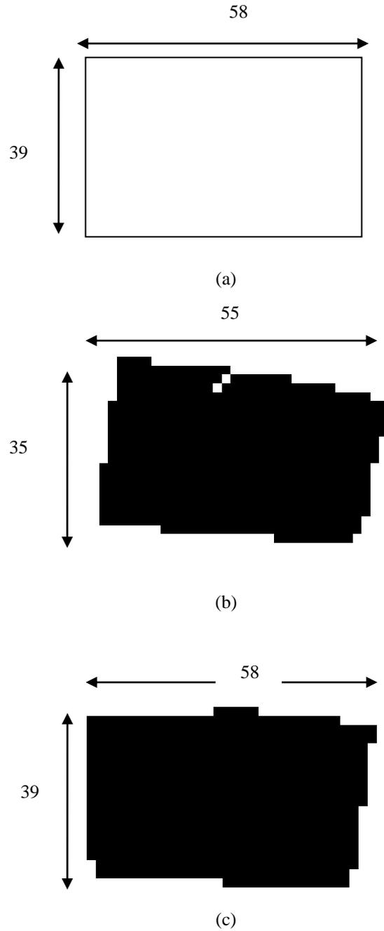
Figure 5: Exploration with real robots. Environment of 37-by-58 cm. (a) is the environment to be explored, (b) is the environment map generated at speed of 300 cm/min, (c) is the environment map generated at speed of 200 cm/minute. The dimensions shown are in centimeters.
