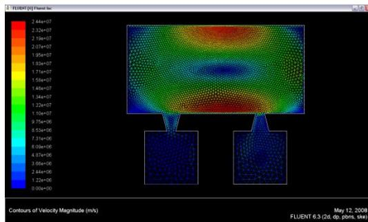
Figure 11. the velocity contour for  $v_{in} = 0$  and actuation= 100Km/s, K- $\epsilon$  turbulent model.
