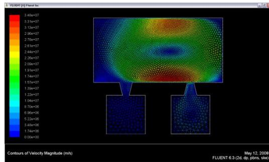
Figure 6. the velocity contour for  $v_{in}$  and actuation of 1000m/s, K- $\epsilon$  turbulent model.
