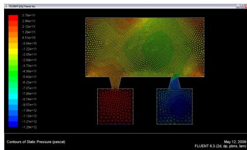
Figure 3. the Pressure contour for  $v_{in}$  and actuation of 1000m/s, laminar.
