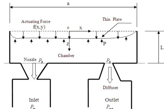
Figure 1. Schematic of the valveless micropump vertical cross section in supply mode.
