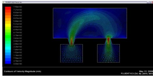
Figure 2. the velocity contour for  $v_{in}$  and actuation of 1000m/s, laminar.
