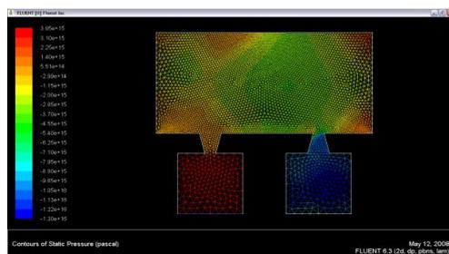
Figure 5. the pressure contour for  $v_{in}$  and actuation of 100 Km/s, laminar.
