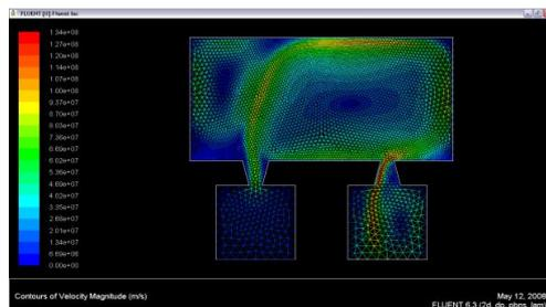
Figure 4. the velocity contour for  $v_{in}$  and actuation of 100 Km/s, laminar.
