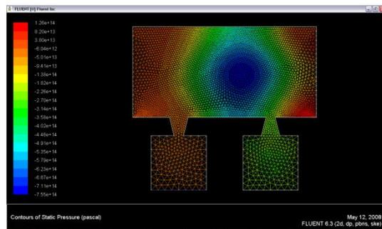
Figure 7. the pressure contour for  $v_{in}$  and actuation of 1000m/s, K- $\epsilon$  turbulent model.
