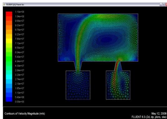
Figure 8. the velocity contour for  $v_{in}$  and actuation of 100Km/s, K- $\epsilon$  turbulent model.
