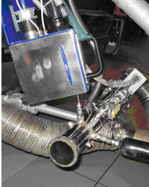
Figure 6. View and diagram of the condensation particle counter [9]
