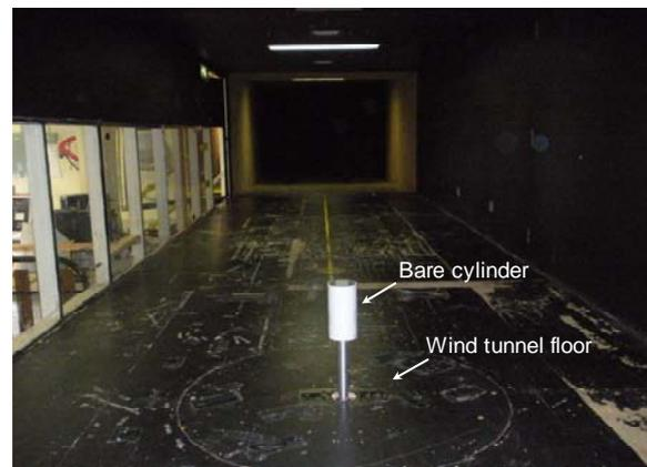
Figure 4. Experimental bare cylinder set up in RMIT Industrial Wind Tunnel
