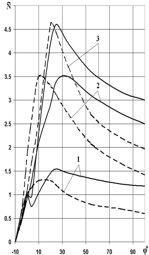
Fig (4) the effect of antismoking additives on soot emission with exhaust gases(rational amount of soot). 1- $Pe=2$ bar 2- $Pe=5$  bar 3- $Pe=7$  bar, \_\_\_diesel fuel, ---- modified diesel fuel, 1300rpm
