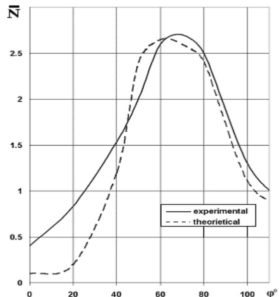
Fig(3) Soot emission with exhaust gases (rational amount of soot). Pe=3bar
