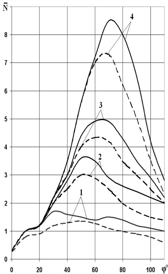
Fig(2) the effect of water emulsification on soot emission with exhaust gases(rational amount of soot). 1- $Pe=1,21$ bar 2- $Pe=2,42$  bar 3- $Pe=3,64$  bar 4- $Pe=4,85$  bar, \_\_\_diesel fuel, ---- Emulsified diesel fuel, 1700rpm
