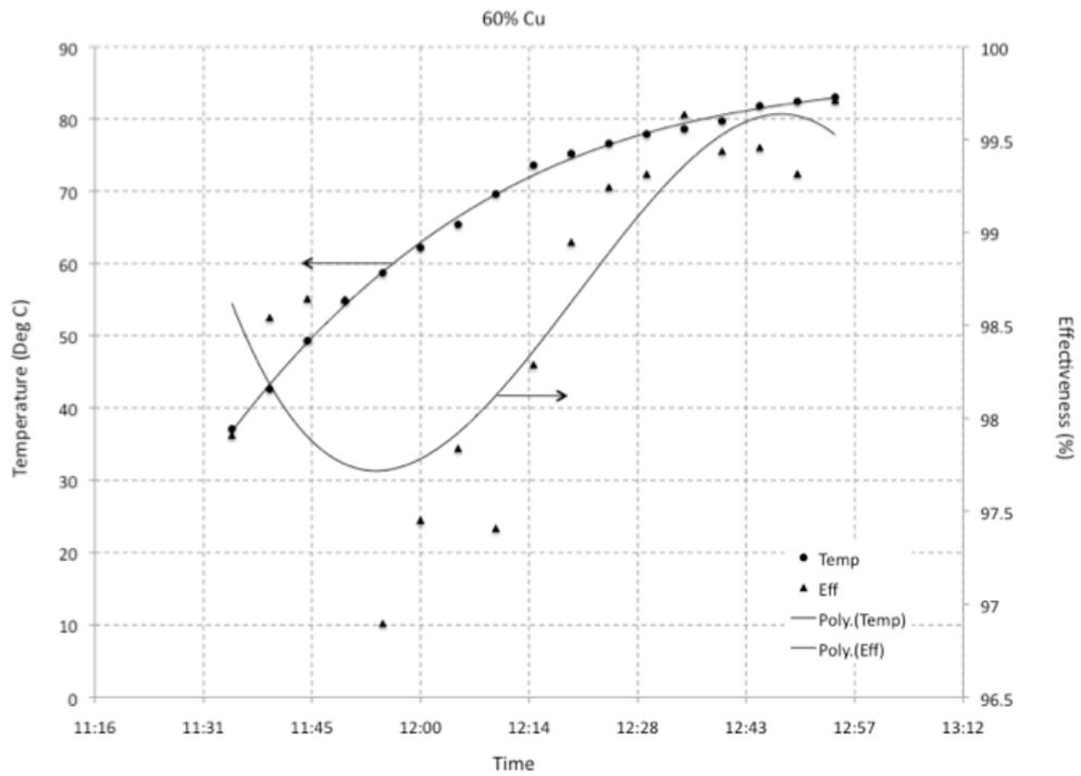
Figure 8 Temperature rise and effectiveness for 60% Cu content
