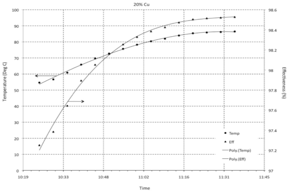
Figure 6 Temperature rise and effectiveness for 20% Cu content
