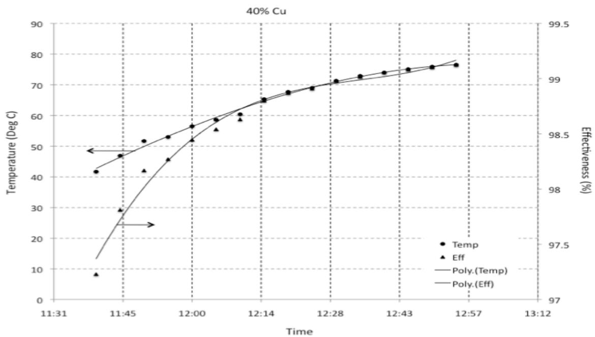
Figure 7 Temperature rise and effectiveness for 40% Cu content
