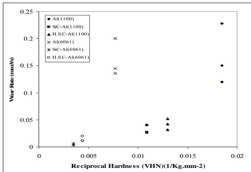
Figure 6. Plots of wear rates versus reciprocal hardness for both Al and Al-alloy matrix composites. With test parameters of; Al<sub>2</sub>O<sub>3</sub> abrasive grit size (250, 180 and 85  $\mu\text{m}$ ), load 10 kg, and sliding speed 180 mm/s.
