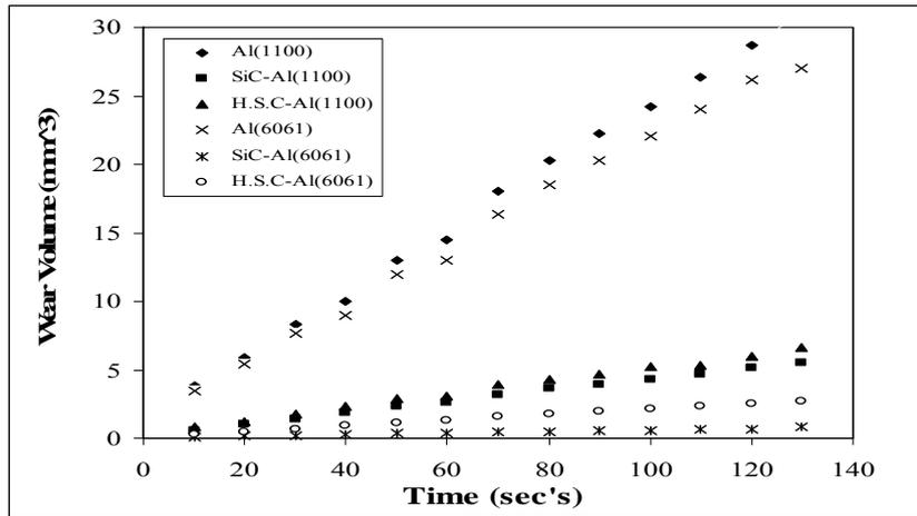
Figure 2. Typical plots of wear volumes versus time to determine wear rates for continuous fibres reinforced and unreinforced Al-matrix composites, with sliding speed 180 mm/s
