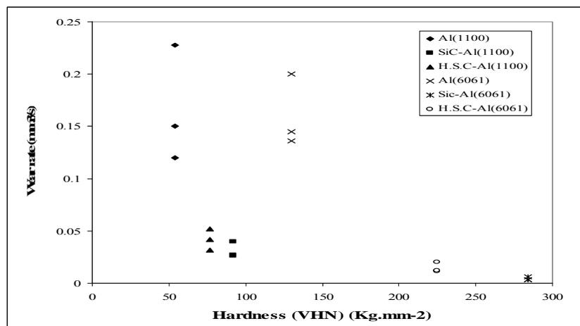
Figure 7. Plots of wear coefficient versus hardness for both Al and Al-alloy matrix composites. With test parameters of; Al<sub>2</sub>O<sub>3</sub> abrasive grit size (250, 180 and 85  $\mu\text{m}$ ), load 10 kg, and sliding speed 180 mm/s.
