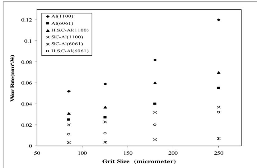
Figure 5. Typical plots of the effect of grit size on wear rates for both continuous fibres Al and Al-alloy matrix composite with test parameters of; load 10 kg, sliding speed 160 mm/s.
