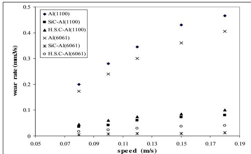
Figure 3. Plots of wear rates versus sliding speed for both continuous fibres Al and Al-alloy matrix composites. With test parameters of; Al<sub>2</sub>O<sub>3</sub> abrasive grit size (250), load 12 kg.
