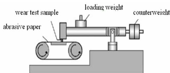
Figure 1. Schematic diagram of abrasive wear testing apparatus.
