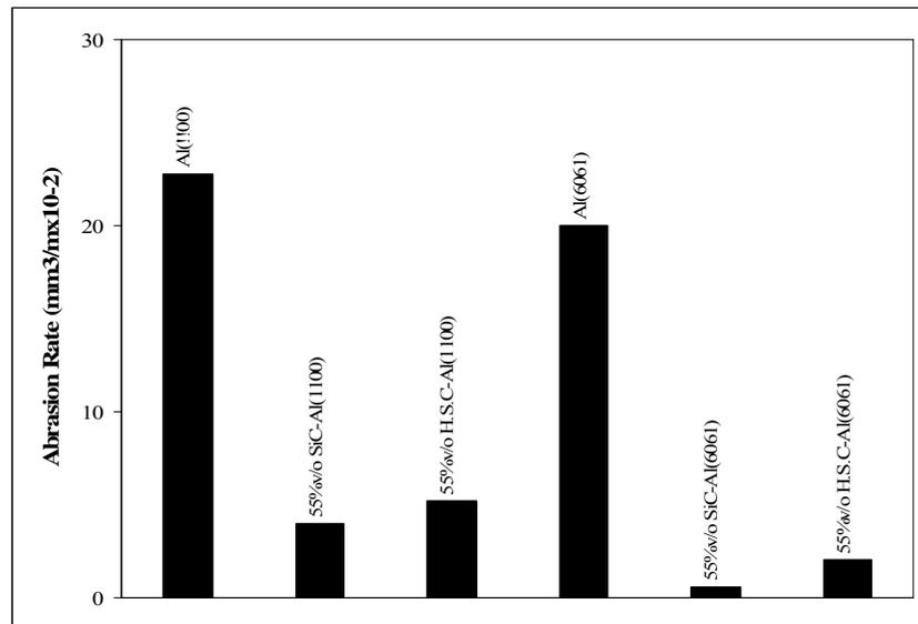
Figure 8. An overall view of, the low stress abrasive wear rates of both continuous fibres Al and Al-alloy matrix composites.
