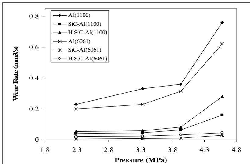
Figure 4. Typical plots of wear rates versus pressure on specimen for both continuous fibres Al and Al-alloy matrix composites. With test parameters of; Al<sub>2</sub>O<sub>3</sub> abrasive grit size (250 μm), sliding speed 180 mm/s.
