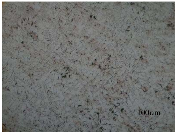
Figure 6. Microstructure at unetched condition.
