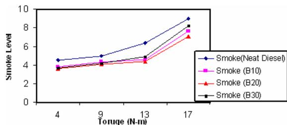
Figure 12. Variation of Smoke Emission with Torque (Engine Speed 850rpm).
