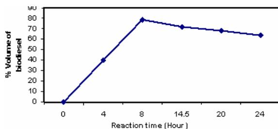
Figure 5. Effect of Reaction Time on Bio-Diesel Production (CH<sub>3</sub>OH=20%NaOCH<sub>3</sub>=0.5%, Reaction Temperature 60°C).
