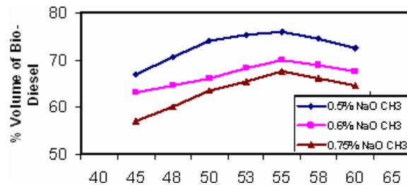
Figure 4. Effect of Catalyst (NaOCH<sub>3</sub>) Percentages on Bio-Diesel (CH<sub>3</sub>OH=20%).
