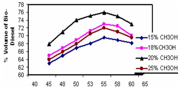
Figure 3. Effect of Temperature on Bio-Diesel Production (NaOCH<sub>3</sub>=0.5%)
