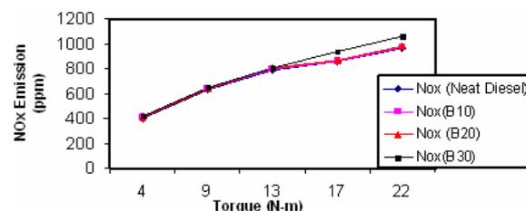
Figure 10. Variation of  $\text{NO}_x$  emission with Engine Torque for Neat Diesel and Bio-Diesel Mixture (engine speed 850 rpm).
