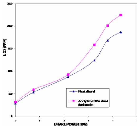
Figure 4. Variation of NO<sub>x</sub> with brake power.
