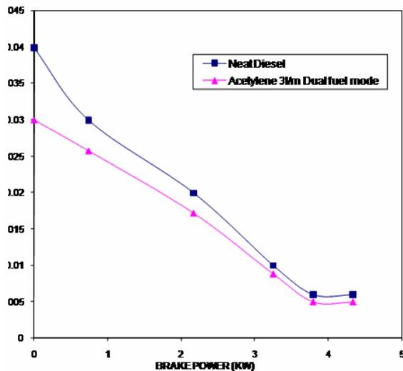
Figure 7. Variation of carbon monoxide with brake power.
