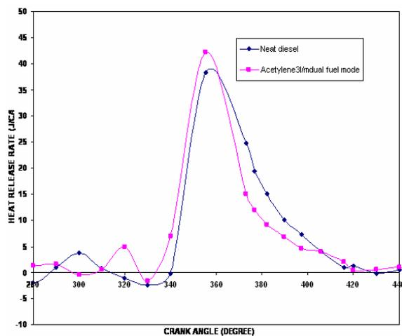
Figure 10. Variation of heat release rate with crank angle .
