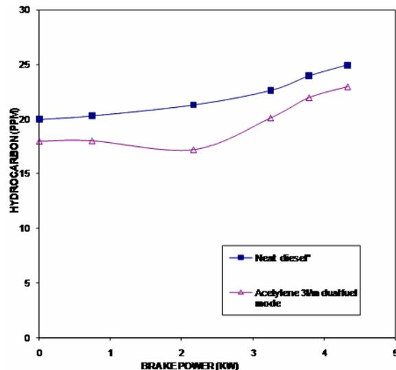
Figure 6. Variation of hydrocarbon with brake power.
