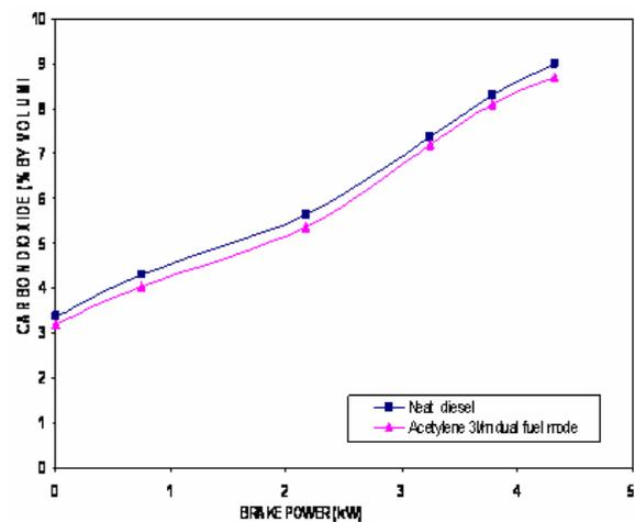
Figure 8. Variation of carbon dioxide with brake power.
