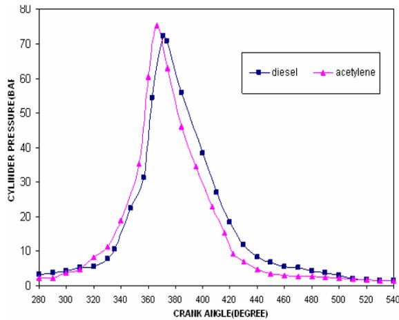
Figure 9. Variation of cylinder pressure with crank angle.
