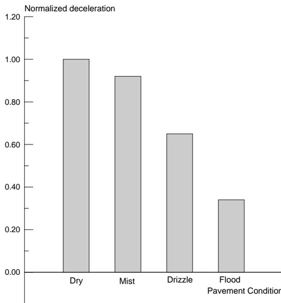
Figure 5. Normalized skid resistance as a function of different wet contact conditions.
