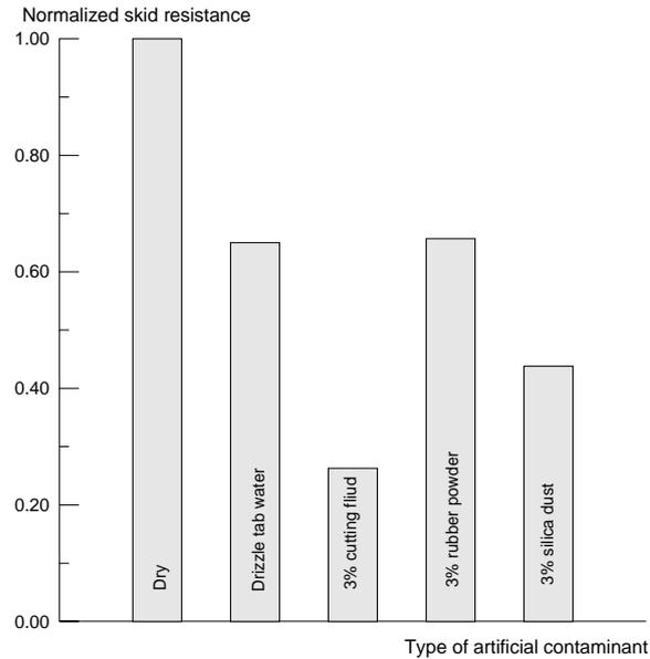
Figure 9. Normalized skid resistance for artificially prepared contaminants .
