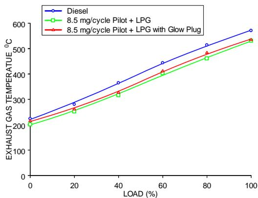
Figure 7 .Variation of Exhaust gas temperature with Load .
