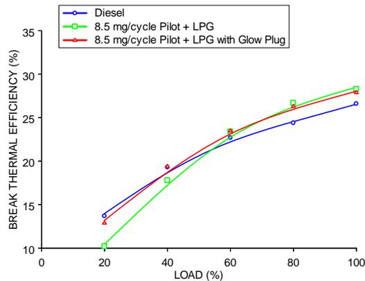
Figure 2 .Variation of Brake Thermal Efficiency with Load.
