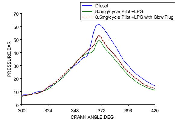
Figure 8. Variation of Pressure with Crank angle at 20 % Load.
