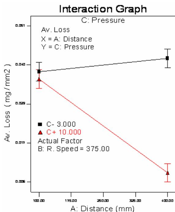
Figure 5. Pressure-Distance interaction effect on average mass loss.
