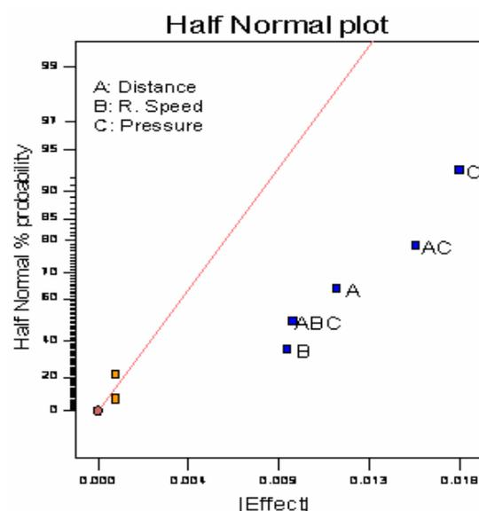
Figure 1. Effects of different factors on the average mass loss.
