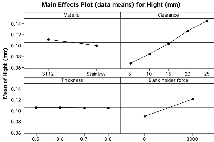
Figure 6. Mean effect plot for bur height
