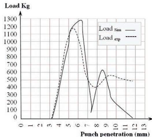
Figure 4. The experimental punch load-penetration curve and the ABAQUS result of the simulated punch load-penetration curve for stainless steel where  $\text{Load}_{\text{simulation}} = 12.75 \text{ kN}$ , and  $\text{Load}_{\text{exp}} = 1200 \text{ Kg} * 9.81 \text{ N/m}^2 = 11.772 \text{ kN}$ .
