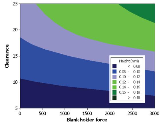
Figure 10. Contour plot of height versus clearance and blank holder force for both materials.
