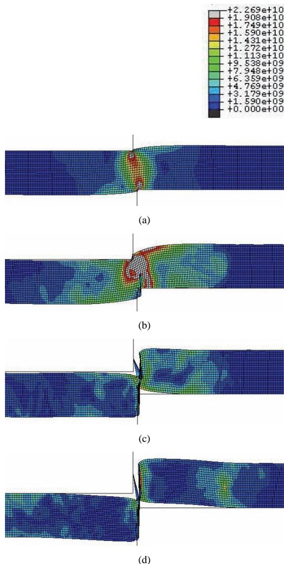
Figure 3. Crack propagation in the mesh for Steel 12
