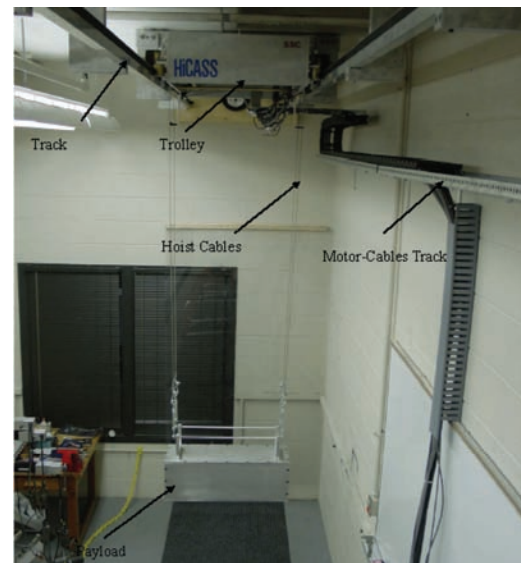
Figure 12: A 1:10 scale model of a 65-ton quay-side container crane
