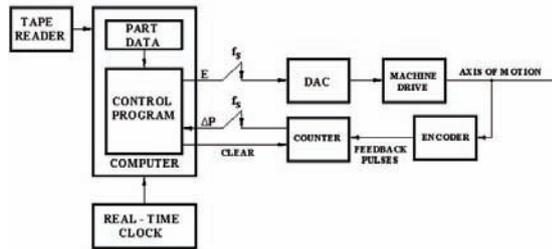
Figure 1: Block diagram of a sampled-data CNC system [4]
