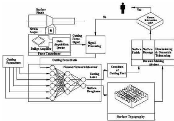
Figure 4: Neural network Monitoring system for turning process [10]
