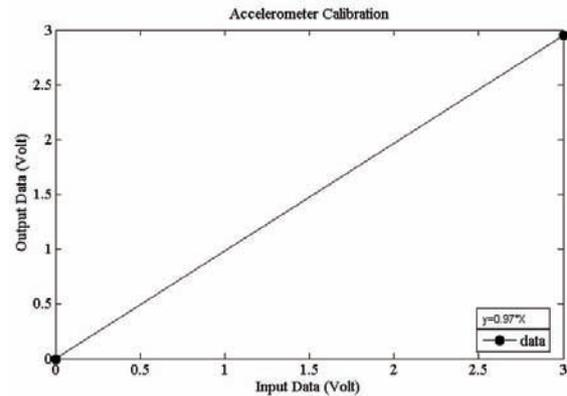
Figure 8: Accelerometer calibration
