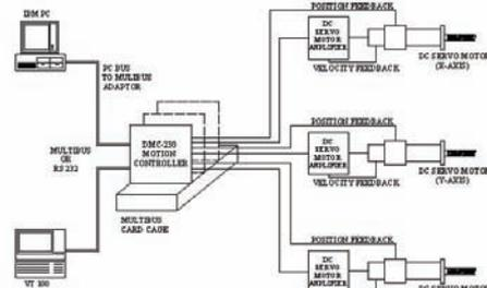
Figure 2: Architecture of speed and position control system for milling process [7]
