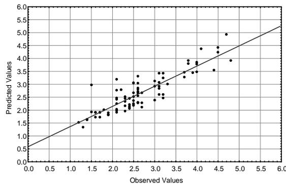
Figure 2: Observed vs. predicted values of surface roughness
