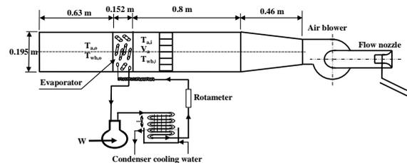
Figure 1: A schematic diagram of the test facility
