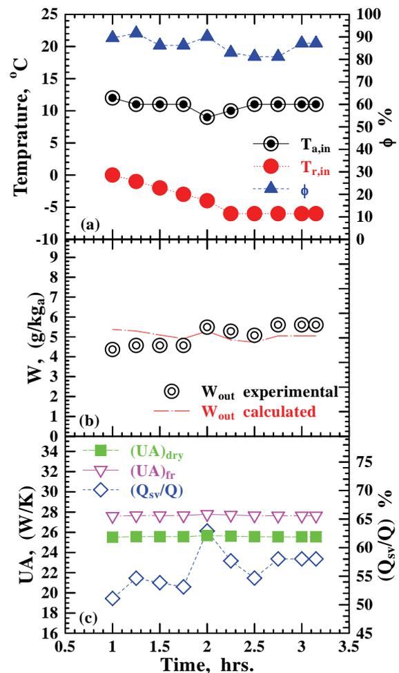
Figure 5: Measured entering operating conditions to the evaporator coil at frost condition (a), the calculated outlet air humidity ratio under frost condition compared with correspondence experimental one (b) and characteristics of the evaporator coil under thin frost formed layer (c)
