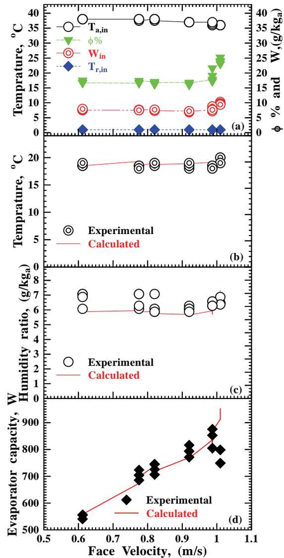
Figure 3: Measured entering operating conditions to the evaporator coil at wet condition (a), comparison of the calculated values with correspondence measured values, outlet air dry-bulb temperature (b), outlet air humidity ratio, (c) and evaporator cooling capacity (d)
