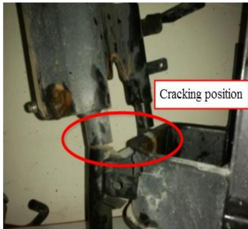
Figure 1. Cracking of urea box bracket
