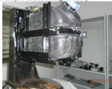
Figure 12. bench test of urea box bracket
