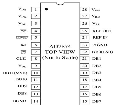
Figure 2. Diagram of AD7874 Pin configuration
