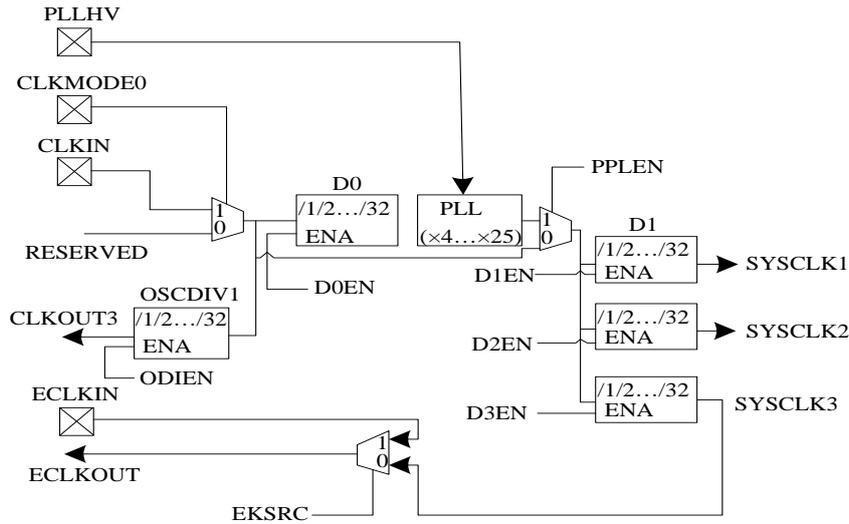
Figure 4. Diagram of clock generation circuit
