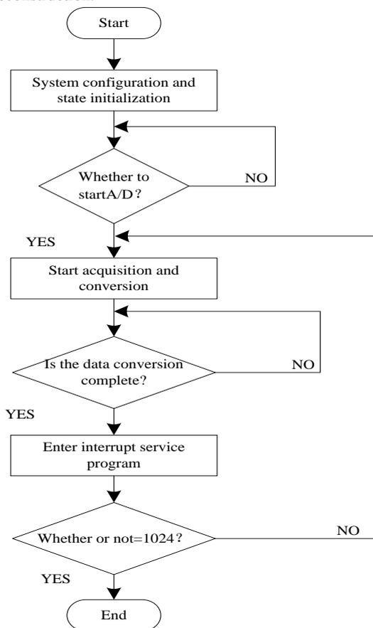
**Figure 6.** Flow chart of program for acquisition and conversion of minor faults signals
