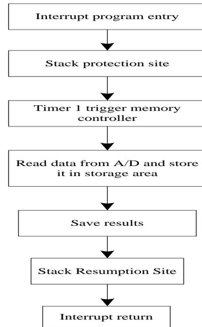
**Figure 7.** Flow chart of sampling interrupt service program for minor fault signal
