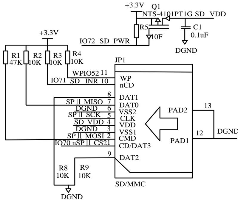
Figure 5. SD memory module circuit
