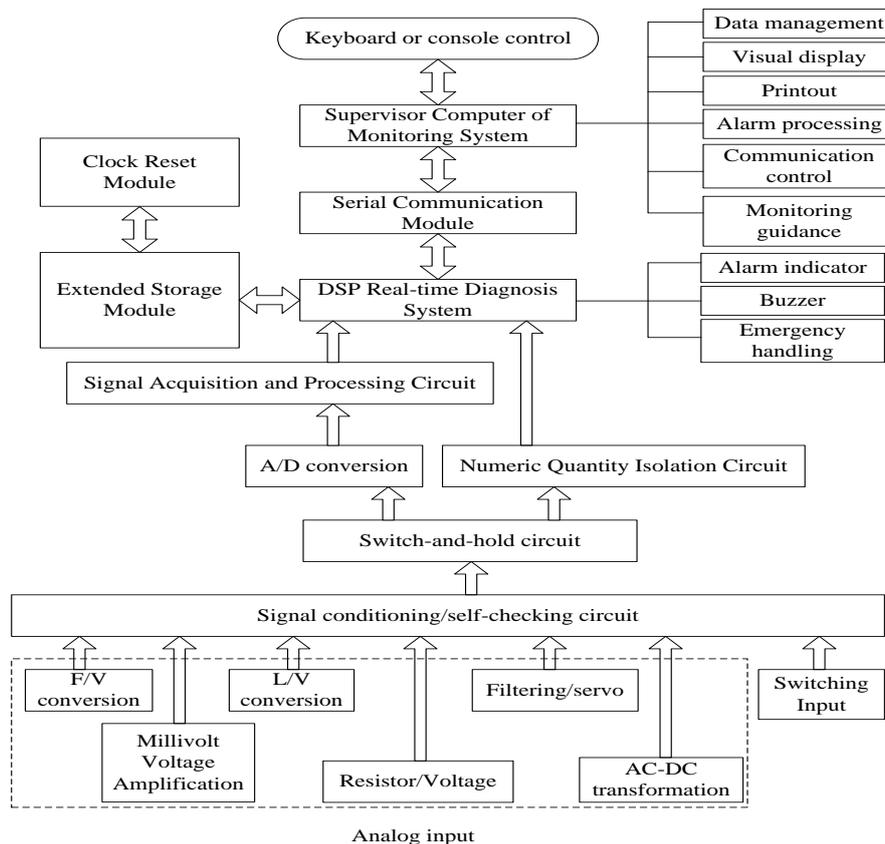
Figure 1. Overall structure of the system
