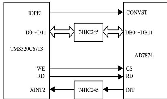
Figure 3. Interface schematic diagram of DSP and AD7874
