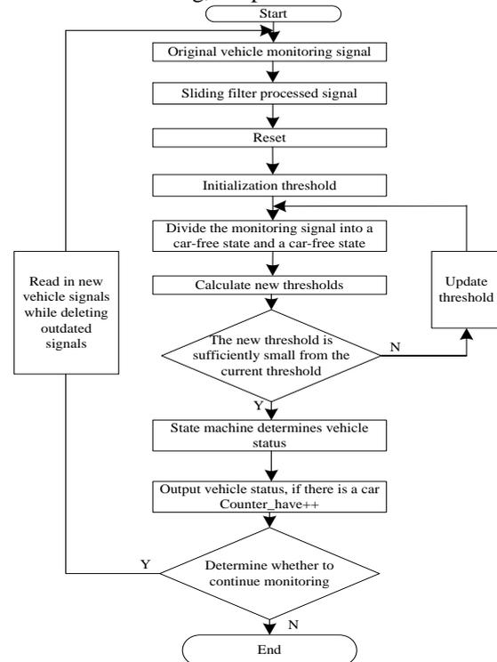
Figure 8. Unmanned vehicle presence algorithm
