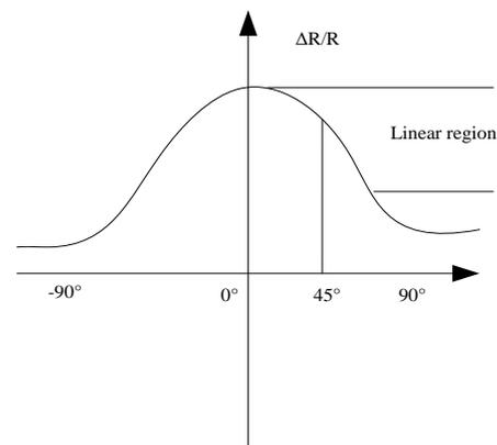
**Figure 1.** Principle of anisotropic magnetoresistance
