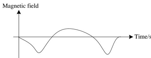
**Figure 5.** Earth's magnetic field curve disturbed by driverless vehicles
