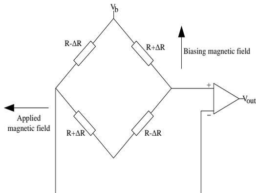
**Figure 2.** Wheatstone bridge magneto-resistive sensor works
