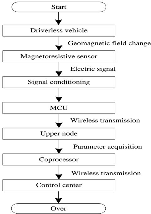
**Figure 4.** Magnetoresistive sensor monitoring speed information of driverless vehicles
