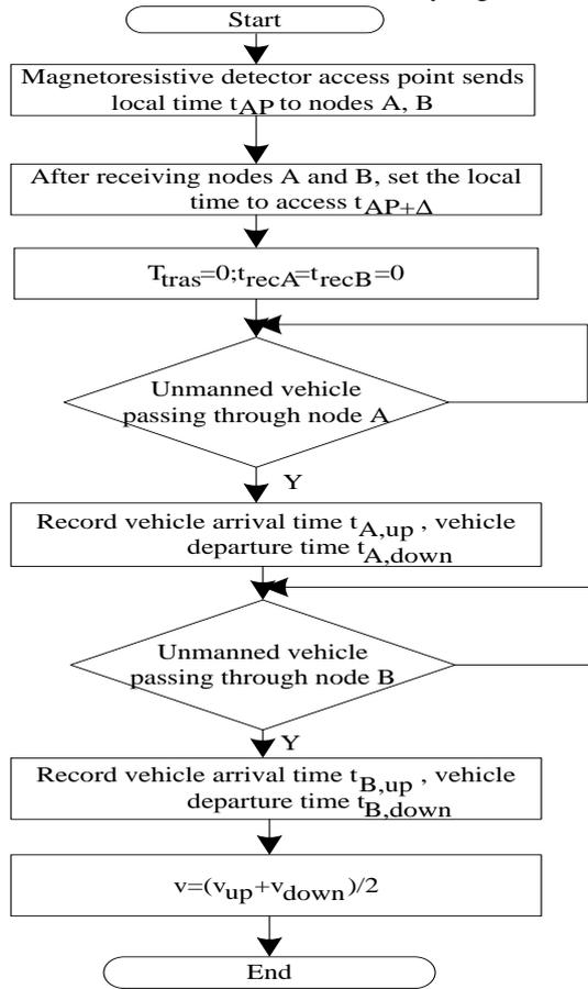
**Figure 9.** Sensor information monitoring algorithm for unmanned vehicles based on magnetoresistive sensor
