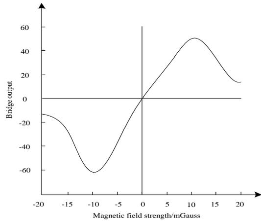
**Figure 3.** AMR magneto-resistive sensor changes with the change of the magnetic field
